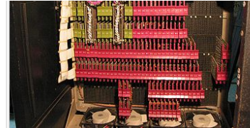
CPU core memory, and external bus interface of a DEC PDP-8/i, made of medium-scale integrated circuits
