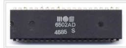
MOS 6502 microprocessor in a dual in-line package, an extremely popular 8-bit design.
