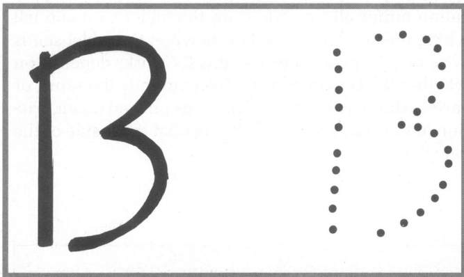
Figure 10. Pen switch pressure sensitivity: Gaps in data due to light writing pressure change a written “B” into “13.”
