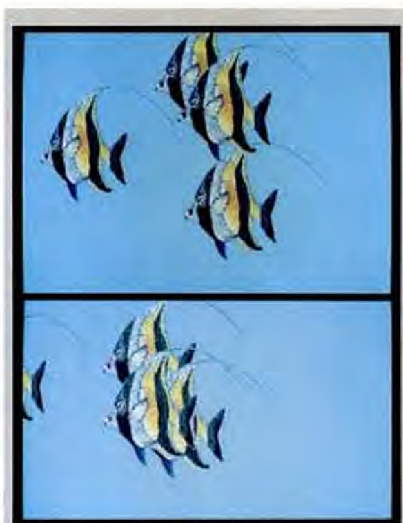
The simplest animation technique—motion across the x-y axis—is made more natural by Animator's spline function. Each of the four fish can travel on a unique track.
