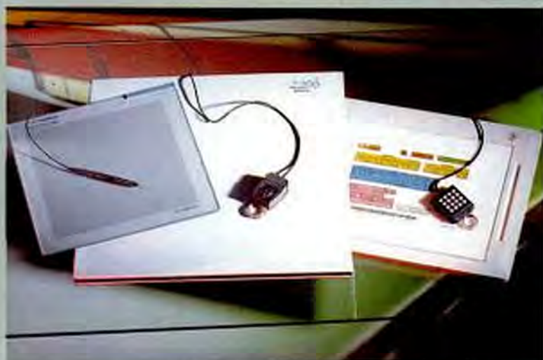
The three tablets representing Numonics' line include (left to right) the $1,395 ZedPEN, the $595 Numonics 2206, and the $595 GraphicMaster. The ZedPEN and the 2206 were once revolutionary products whose practicality and ergonomics have waned in comparison with the evolutionary, sleek, and upwardly mobile GraphicMaster.
