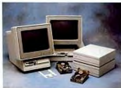
IBM® PS/2 Models 25, 30 and 30-286 Solutions: (Internal) 20, 30 and 40 MB; 40-24 ns. (External) PC Stack: 30, 45 and 80 MB; 40-28 ns.
