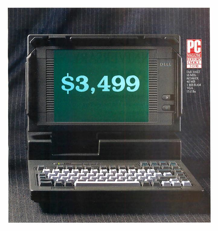
The laptop above is ours. The Dell<sup>\*\*</sup> 316LT. It comes with an Intel<sup>®</sup> 386'\*SX CPU running at 16 MHz. 1 MB of RAM, expandable to 8 MB, and a backlit VGA display. With a 40 MB hard drive it weighs 15 lbs. It won the *InfoWorld* Exceptional Value Award, and was one of only two 386SX laptops to win the *PC Magazine* Editor's Choice Award.
