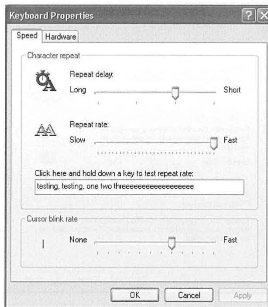
Figure 8-15: How fast do you want your keys to repeat? This control panel also offers a Hardware tab, but you won't go there very often. You'll use it exclusively when you're trying to troubleshoot your keyboard or its driver.
