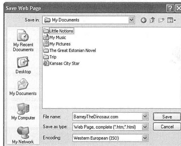
Bottom: The buttons at the left side of the Save As dialog box provide quick access to the folders where you're most likely to stash newly created documents: the My Documents folder, the desktop itself, and so on. But by using the "Save in:" drop-down list at the top of the screen, you can choose any folder you like.
