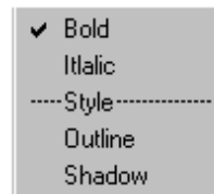
Figure 7.6 Inappropriate use of a separator
