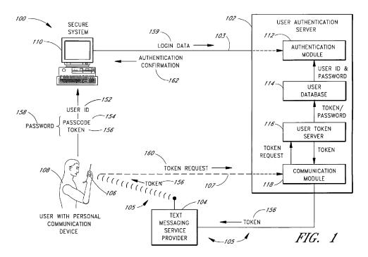
The patent teaches a system with similar benefits without requiring the user to carry such a card. As shown in FIG. 1 (above), a token server (116) running on a user authentication server (102) generates a random token in response to a user request (160) for a new password. The server (102) creates the new password based on a secret passcode known to the user and the to-
