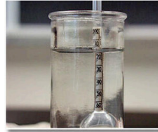
Sources/Usage: Public Domain. View Media Details A hydrometer is used to measure density of liquid.
