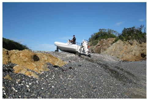
For easier maneuvering with AWD activated, Sealegs runs in limited slip mode which makes the craft very capable in most situations. When maximum traction is required, a quick push engages full diff lock mode. This allows all driving wheels to turn at the same rate for reduced wheelspin and is generally only required for a few seconds when climbing over a beach li
