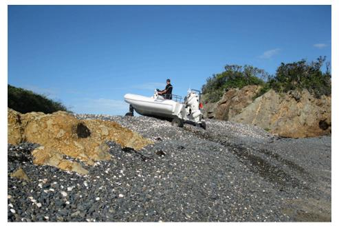
For easier maneuvering with AWD activated, Sealegs runs in limited slip mode which makes the craft very capable in most situations. When maximum traction is required, a quick push engages full diff lock mode. This allows all driving wheels to turn at the same rate for reduced wheelspin and is generally only required for a few seconds when climbing over a beach lip
