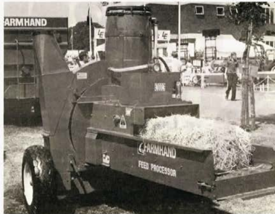
The Farmhand caustic soda applicator is mounted on a basic Farmhand Feed Processor which requires at least 85 tractor hp. Soda solution is metered by a roller vane pump as straw enters the Processor. For more details, contact: FARM SHOW Followup, Farmhand, Inc., 1011 South 1st St., Hopkins, Minn. (ph. 612 938-7651).
