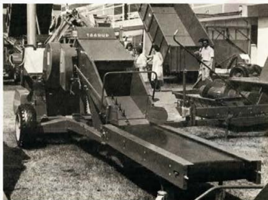
The Taarup Straw Processor has a capacity of 2-2½ tons per hr. and requires a 100 hp tractor. Caustic soda solution is applied as straw leaves the grinder. A series of spiked rotors massages the solution into the straw. For more details, contact: FARM SHOW Followup, Maskinfabrikken Taarup A/S, 5300 Kerteminde, Denmark.
