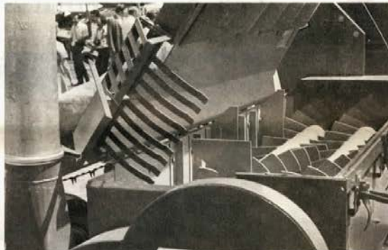
The JF straw processor requires about 70 pto hp and applies caustic soda solution as straw leaves the hammermill-type grinder. "Hard-mixing" occurs in the mixing chamber where liquid is rubbed into the straw by a beater-type mixer. Capacity is 2-2½ tons per hr. For more details, contact: FARM SHOW Followup, Terry Grace, Farmax, Box 8523, Mobile, Ala. 36608 (ph. 205 479-8663).
