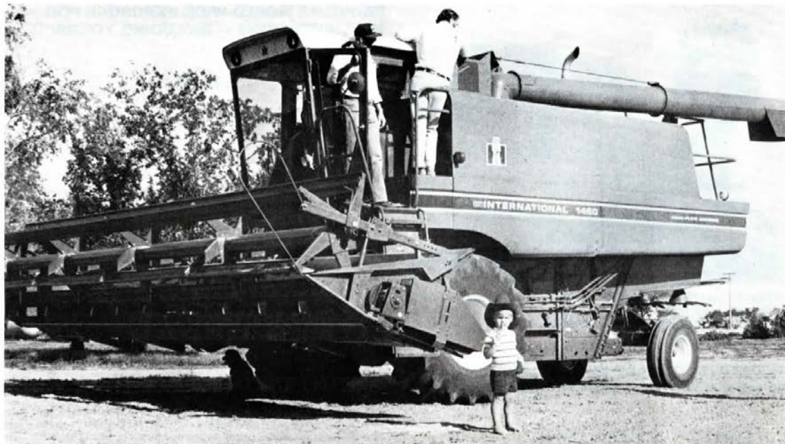
Les Renner reports that his new IH "rotary" has no cylinder or straw walkers.
