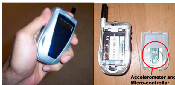
Figure 1: Prototype of a Motorola i95c1 instrumented with a 2-axis accelerometer.
