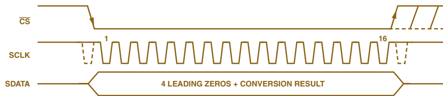
Figure 2. Serial interface signals in a normal conversion.
