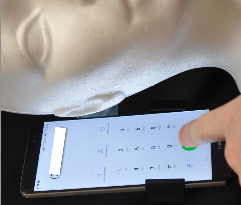
The second image shows that, after the call button is pressed and the ear is proximate to the Huawei Mate 9, power to the display is reduced and the display is darkened.
