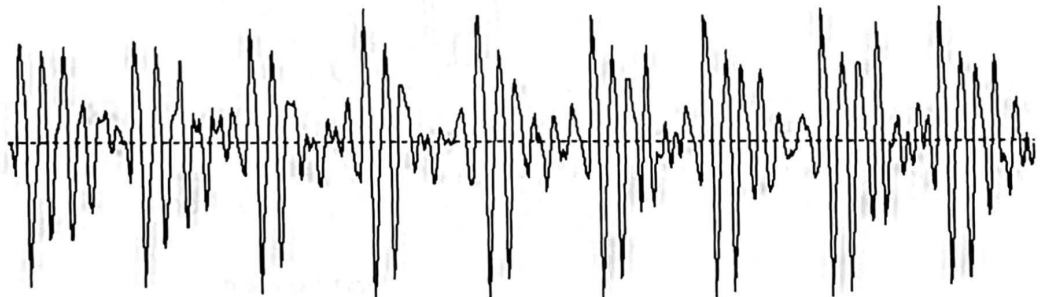
Figure 2.6. A waveform of the vowel in "but." The display shows amplitude mapped against time, over a 100 millisecond interval. Nine pitch periods can be seen; the frequency of voicing is about 90 Hz.
