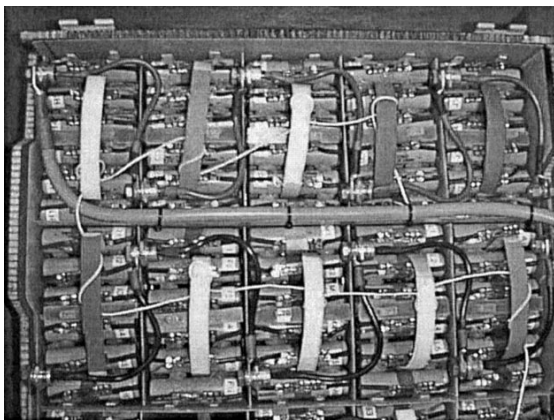
Fig. 4. Ten Li-ion modules viewed from above (bypass diodes shown on top of cells).
