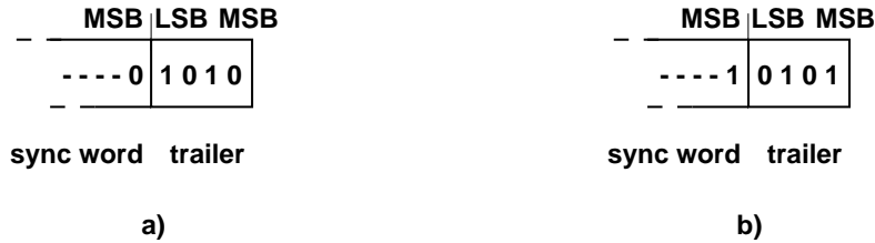
Figure 18—Trailer in CAC when MSB of sync word is 0 (a), and when MSB of sync word is 1 (b)
