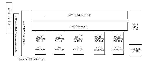
This family of standards deals with the Physical and Data Link layers as defined by the International Organization for Standardization (ISO) Open Systems Interconnection (OSI) Basic Reference Model (ISO/ IEC 7498-1: 1994). The access standards define five types of medium access technologies and associated physical media, each appropriate for particular applications or system objectives. Some access standards have been withdrawn and other types are under investigation.
