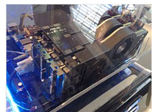
3-way GeForce 8800 Ultra in an SLI using a rigid bridging connector
