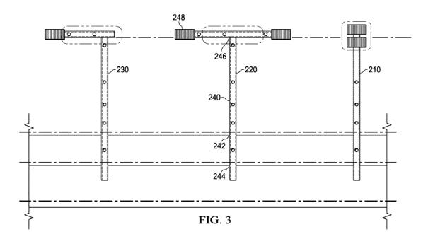
Figure 3 above shows light units 210, 220, and 230, which may include mounting pole 240, bracket for a top rail 242, bracket for a bottom rail 244, cap 246, and light fixture 248. *Id.* at 2:63–65. The bracket for top rail 242 and bracket for bottom rail 244 may be used to attach light mounting pole 240 to rails 205 of a crown deck (dashed lines) of a drilling rig using U-shaped bolts or straps. *Id.* at 2:63–3:1.
