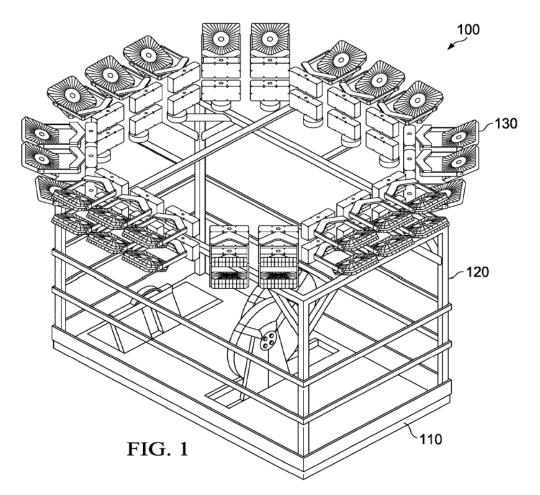
Figure 1 above shows a prior art lighting system 100 built from a single frame 120, which includes multiple frame lights 130 rigidly fixed onto the frame 120. *Id.* at 2:25–29. The '016 patent explains that "frame 120 may be installed on the crown 110, or top, of a drilling rig such that the ground around the drilling rig is illuminated when in use." *Id.* at 2:30–32.
