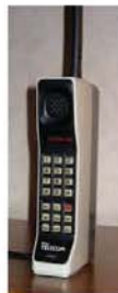
Weighing in at 2 pounds, the Motorola DynaTac provided 30 minutes of talk time and took roughly 10 hours to charge.
