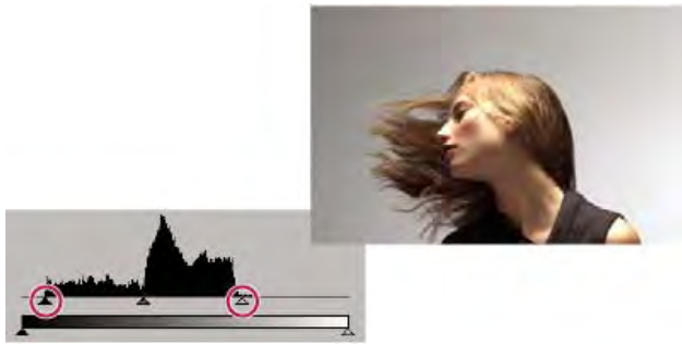
Input sliders moved so that output uses full tonal range
