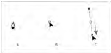
Drawing the first vertex in a curved path
