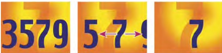
Animating the tracking values for the characters 3579 (left and center) so that only the 7 in the middle remains (right)
