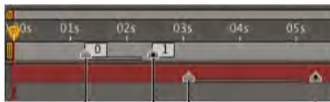
A. composition marker with duration of 1 second B. composition marker with cue-point data C. layer marker with duration of 2 seconds D. layer marker with cue-point data
