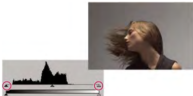
Histogram for image that does not use full tonal range
