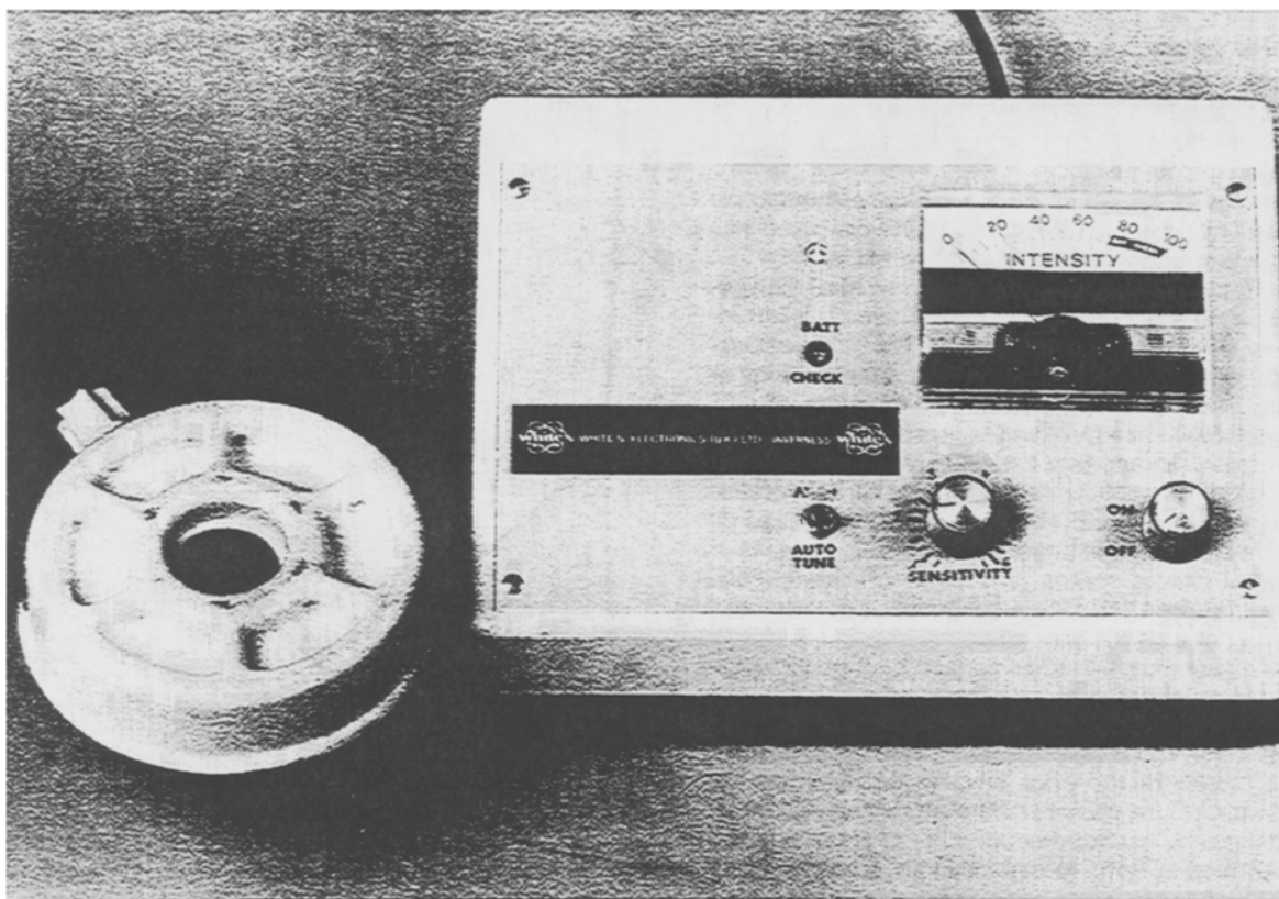
Fig 1. Metal detector EAS II with plate-shaped probe. A tuner allows for compensation of the metal content of the surroundings. The sensitivity adjustment modifies the intensity of the signal. It permits measurements in the optimal range of the scale and to calculate the distance of the metal particle to the probe.
