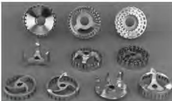
Figure 39-4. Types of rotors used in colloid mills. These may be smooth (for most emulsions), serrated (for ointments and very viscous products), or of vitrified stone (for the paints and pigment dispersions) (courtesy, Tri-Homo).
