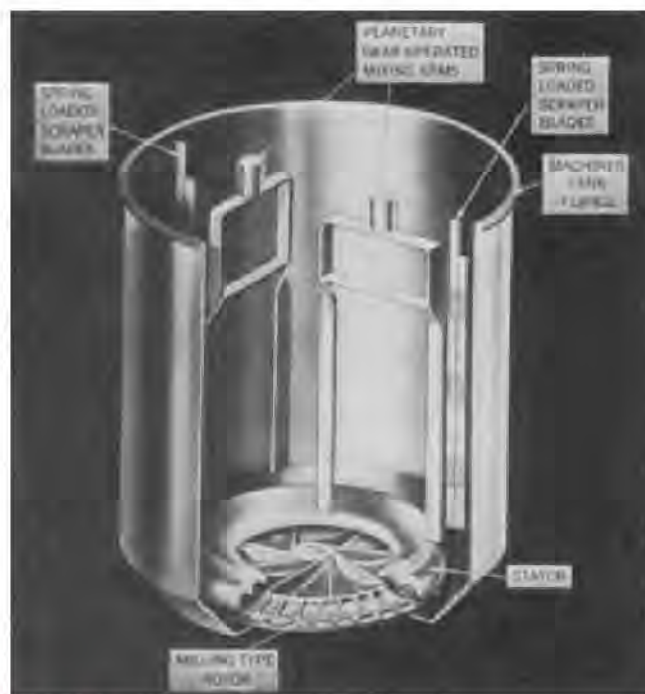
Figure 39-2. Standard paste-type dispersal mixer with cupped-rotor milling element and double-rotating mixing arm circulating element (courtesy, Abbe Eng).
