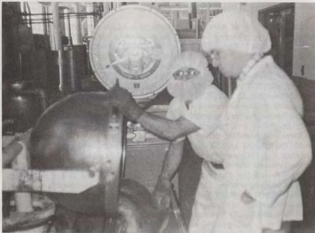
Figure 27 Completed candy base being transferred to weighing container. All batch weights are double-checked. (Warner-Lambert Co.)
