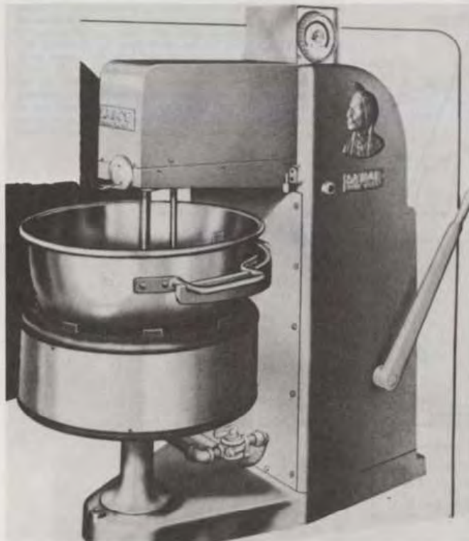
Figure 11 Atmospheric gas furnace. Features: single or double action agitation with scraping action; 30 to 60 rpm stirring speed; thermostatic control; 110,000 to 286,000 BTU heat output; removable agitator; copper kettle 24 in. \times 12 1/2 in. \times 16 in. deep. (Savage Brothers Co., Elk Grove Village, Ill.)
