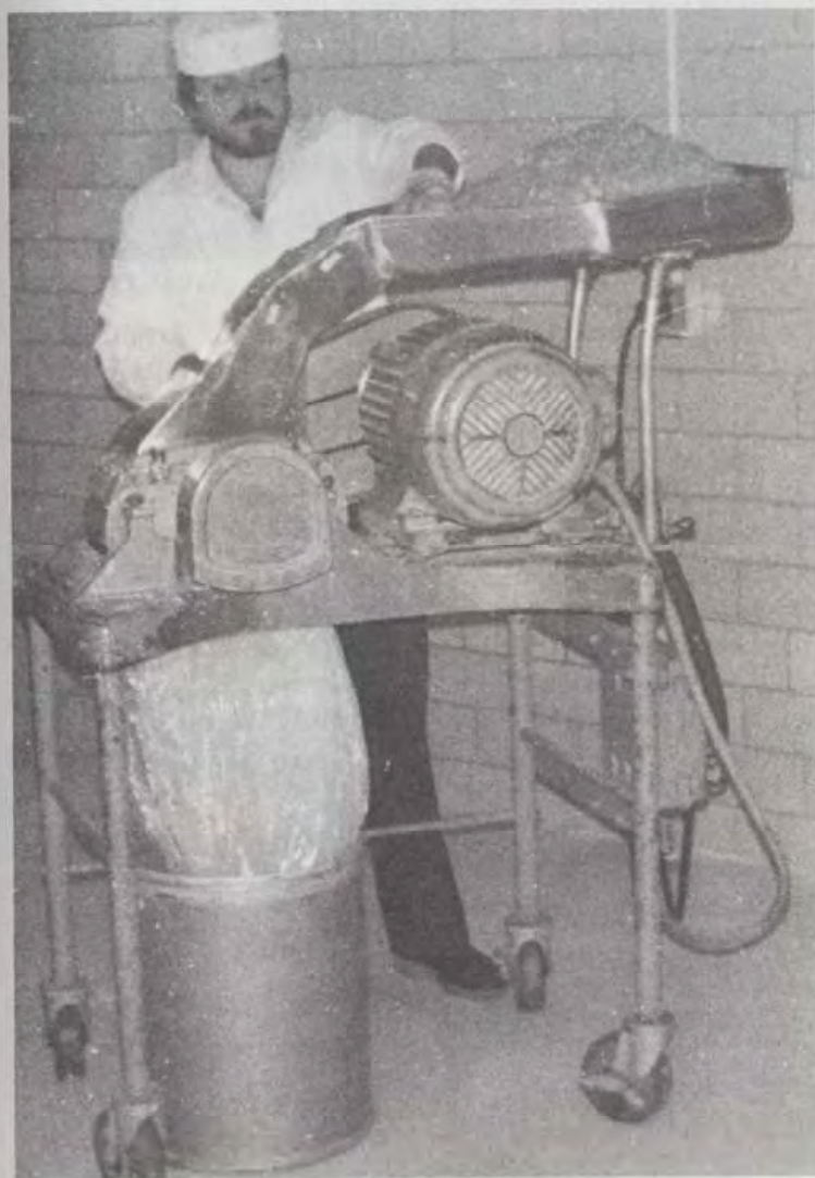
Figure 36 Lozenges rejected due to manufacturing difficulties are milled to a particle size range of 20 to 50 mesh. This produces granules that will absorb the liquid-flavor mixture, to prevent flavor and medicament segregation during medicament-flavor premix preparation and storage. (Warner-Lambert Co.)
