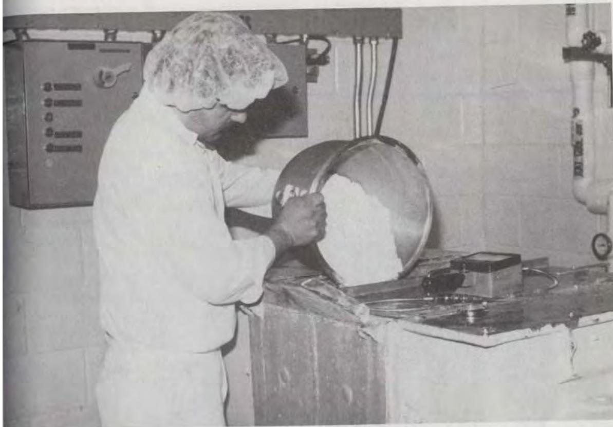
Figure 80 Flavor and seeding crystal addition. Seed should not be mixed for more than 10 minutes to avoid melting of the seed crystals into the batch. (Warner-Lambert Co.)
