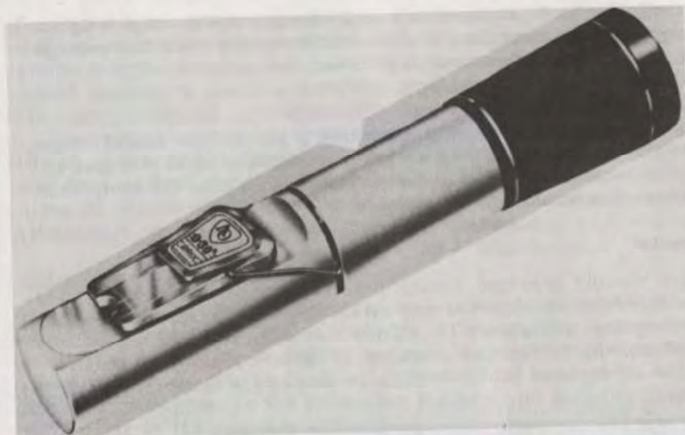
Figure 98 Hand refractometer. Designed for rapid field-determination of dissolved sugar content. The instrument automatically compensates for temperatures from 16 to 38°C. (American Optical Co.)
