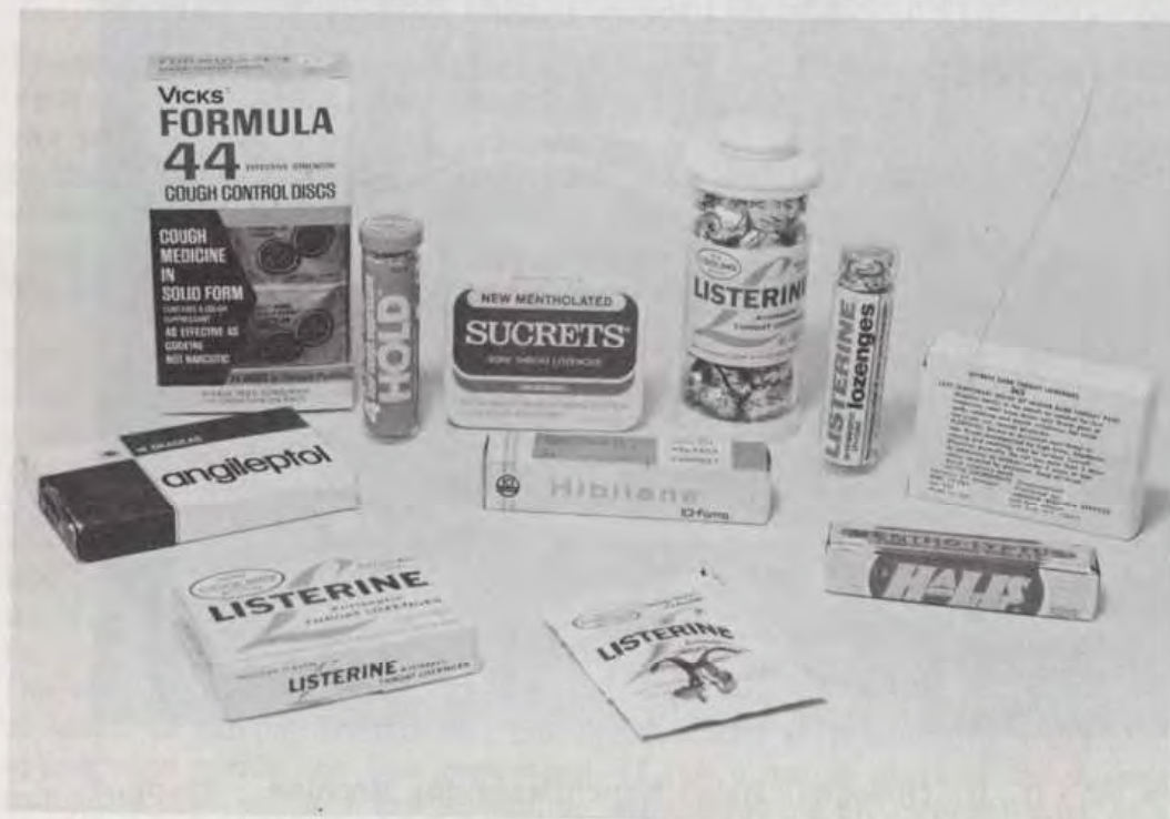
Figure 71 Production trade packages. Cardboard box, foil pouch, styrene tube, metal box, strip-pack, and roll are the most common in use.
