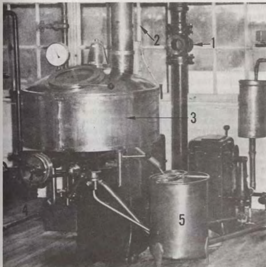
Figure 17 Precooker for production of 650 to 2750 pounds of sugar plus glucose per hour. (1) Corn syrup line; (2) liquid sugar line; (3) precooker; (4) syrup flow valve; (5) intermediate holding container. (Robert Bosch GmbH, Div. Hamac-Höller.)
