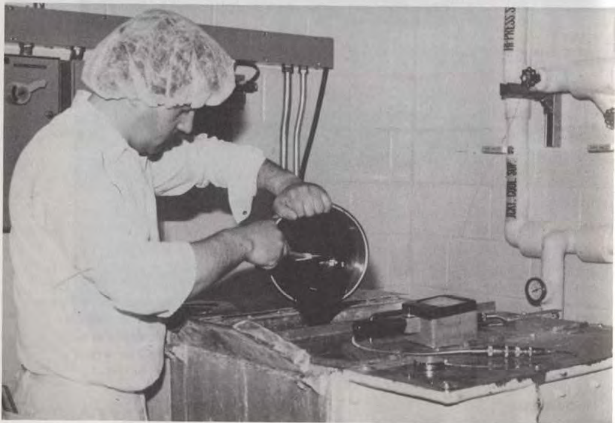
Figure 78 Color addition. Dyes are suspended in propylene glycol or glycerin to aid distribution. (Warner-Lambert Co.)
