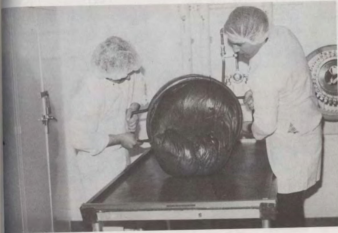
Figure 82 Medicated caramel base is deposited onto a cooling table. During this rapid cooling period a product with a coarse grain is formed. At least 3 to 4 hours cooling is required to enable the product to properly grain before extrusion. (Warner-Lambert Co.)
