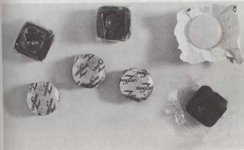
Figure 67 Individually bunch wrapped lozenges. Laminated aluminum foil or cellophane wraps are most commonly used.
