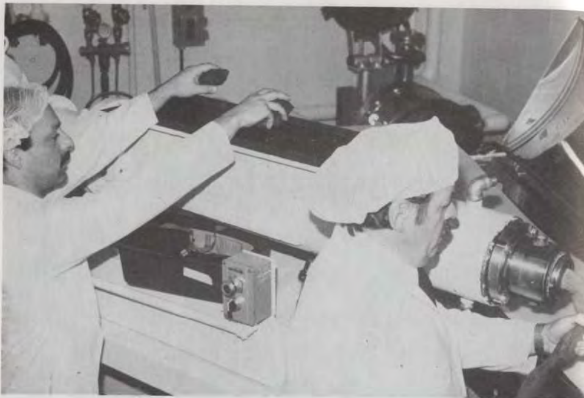
Figure 84 Grained caramel mass is extruded into a flexible candy rope. Diameter and shape of the rope can be adjusted by changing the exit die configuration. (Warner-Lambert Co.)
