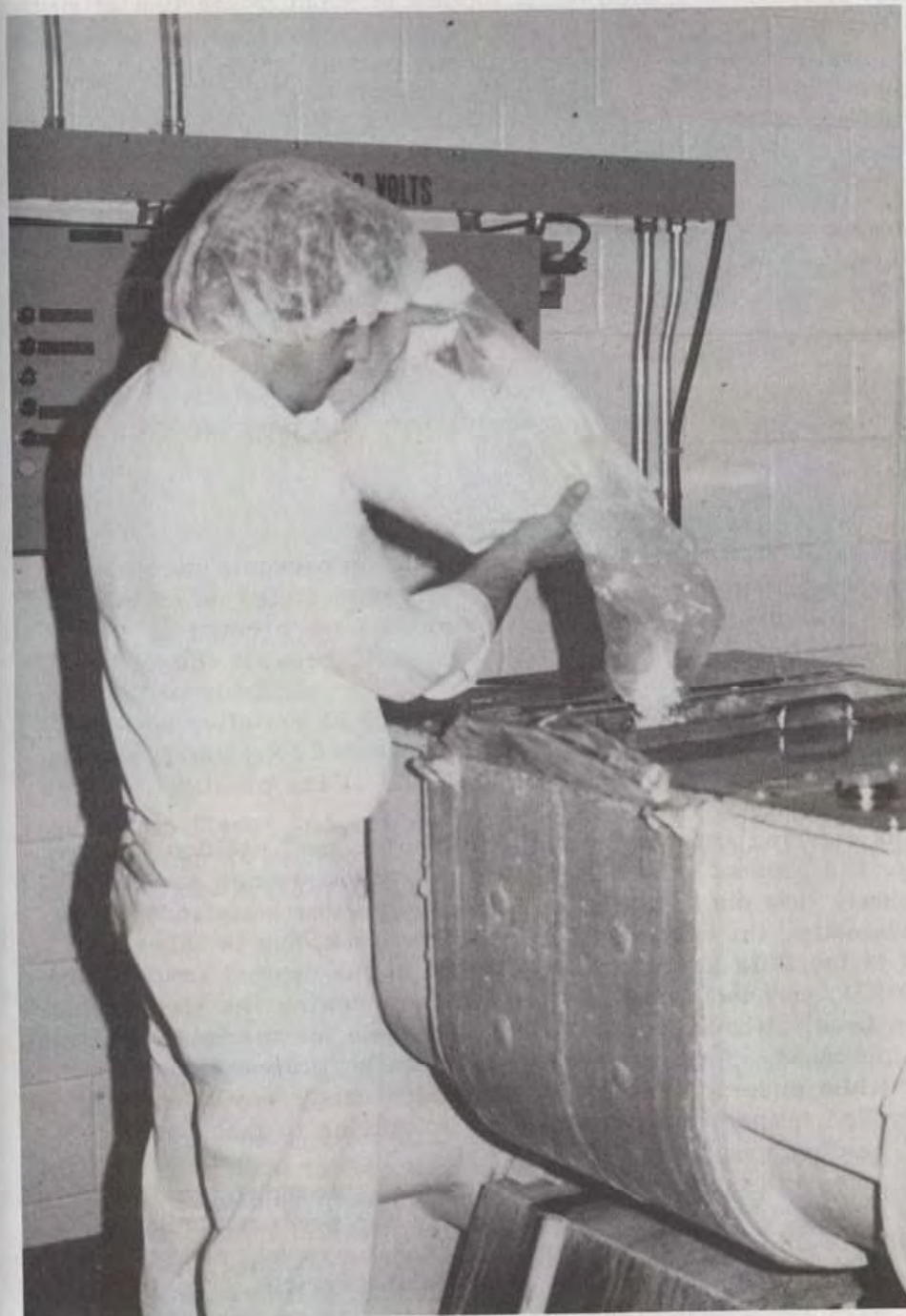
Figure 79 Medicament addition. Heat stability of the drugs determines at what temperature they may be added. (Warner-Lambert Co.)
