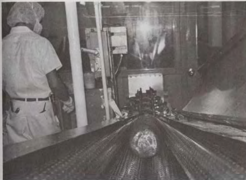
Figure 39 Candy base after forming is fed into sizing rollers from batch former. Note that candy mass has been formed into a cylinder. (Warner-Lambert Co.)
