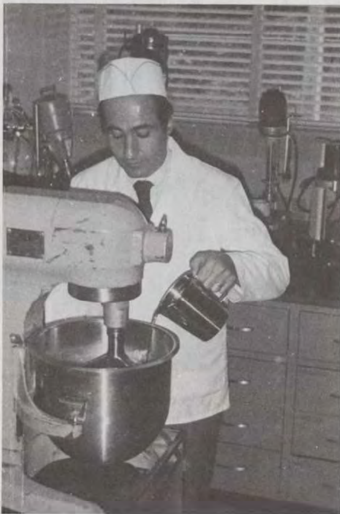
Figure 33. Preparation of flavor, medicament, and ground salvage mixture on an individual batch basis. Sufficient material is contained in the premix for incorporation into 100 lb. of cooked candy base. This procedure can be used to prepare experimental as well as production batches. Here the flavor is added to the ground salvage and medicament mixture. (Warner-Lambert Co.)
