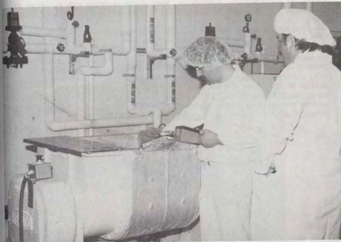
Figure 77 Candy base is mixed to a temperature below 120^{\circ}\text{C} . At this point the whipping agents may be added. (Warner-Lambert Co.)
