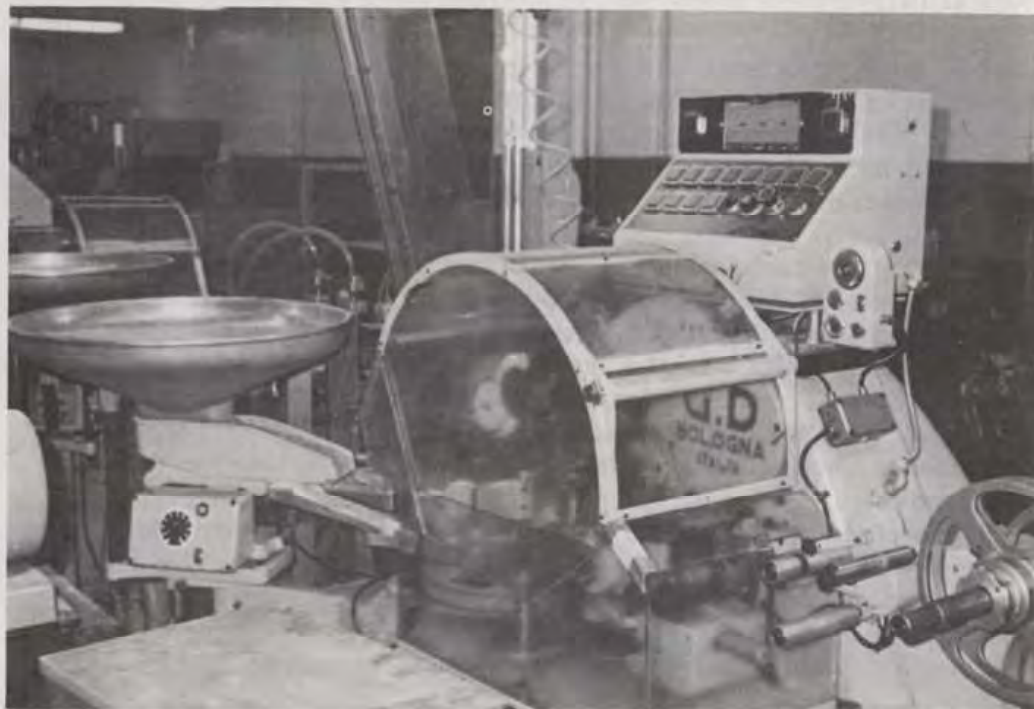
Figure 68 G. D. (Bologna, Italy) lozenge bunch wrapping machine. Unwrapped lozenges are stored in the hopper prior to mechanical aligning and passage into the bunch wrapping machine. (Warner-Lambert Co.)
