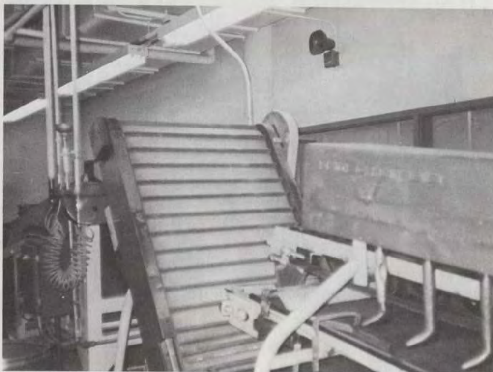
Figure 56 Cooled lozenges are transferred to an elevator for movement to the sizing rollers. (Warner-Lambert Co.)
