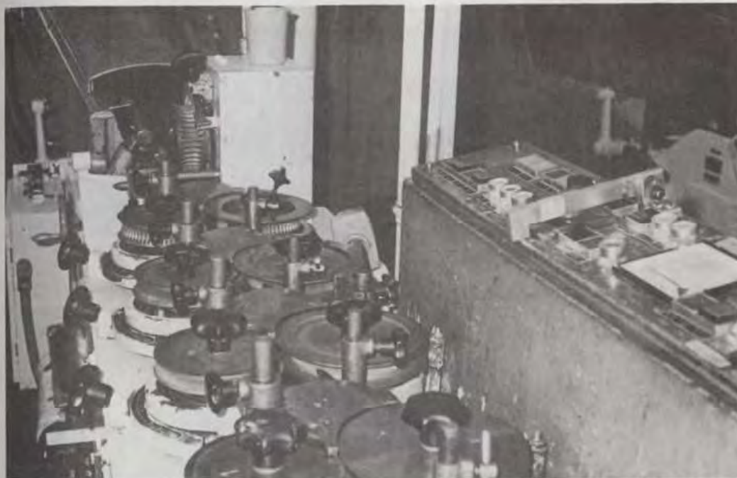
Figure 42 Candy rope is fed through the sizing rollers. Diameter of candy rope determines final lozenge weight. (Warner-Lambert Co.)
