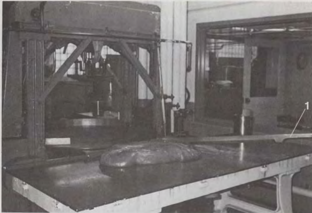
Figure 37 Mixed candy base on tempering table prior to batch forming. Cutting blade on right (1) is used to cut the mass into equal portions for ease of handling. (Warner-Lambert Co.)
