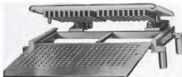
Figure 45-34. Tablet triturate mold (courtesy, Vector/Colton).
