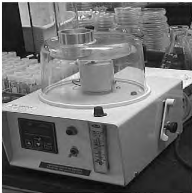
Figure 41-14. Example of slit-to-air sampler (courtesy, Baxter).
