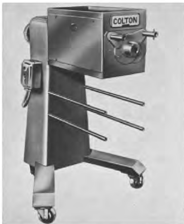
Figure 45-10. Rotary granulator and sifter (courtesy, Vector/Colton).
