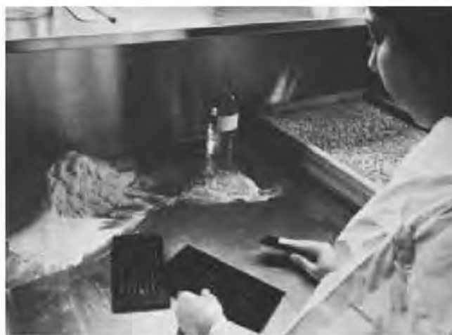
Figure 45-33. Hand-molding tablet triturates (courtesy, Merck).
