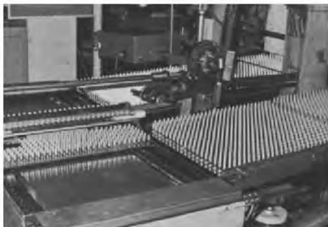
Figure 45-41. Formed capsules being dried by rotating through a drying kiln (courtesy, Lilly).
