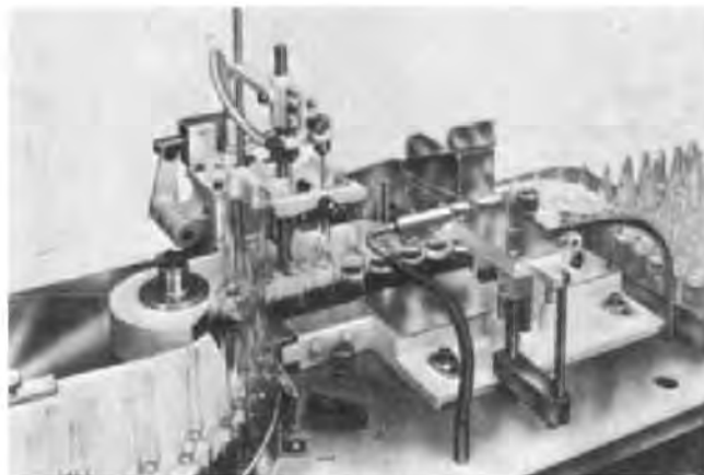
Figure 41-24. Automatic filling and pull-sealing of ampoules (courtesy, Cozzoli).
