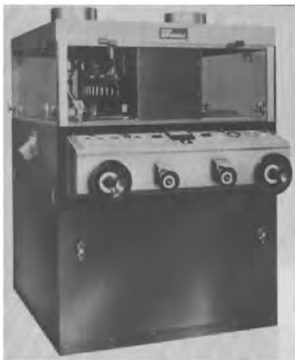
Figure 45-22. Model 747 High Speed Press, double-sided rotary compacting press designed to produce at speeds over 10,000/min (courtesy, Stokes/Pennwalt).
