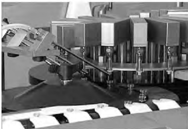
Figure 41-25. Mechanical device for inserting rubber closures in vials (courtesy, Baxter).
