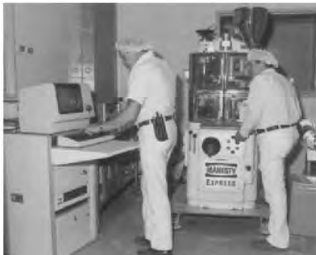
Figure 45-24. Research technicians use an instrumented tablet press to develop processes at Schering-Plough.
