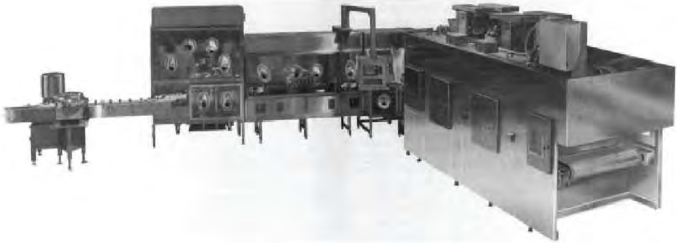
Figure 41-11. Large-scale production line showing, from right to left, container-sterilizing tunnel feeding into isolator enclosing filling and sealing, with access glove ports, and exiting to capper (courtesy, TL Systems).
