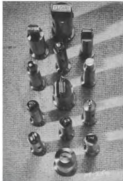
Figure 45-19. Collection of punches (courtesy, Stokes/Pennwalt).
