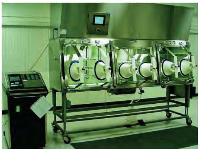
Figure 41-32. Example of an isolator used for sterility testing (courtesy, Baxter). See Color Plate 18.
