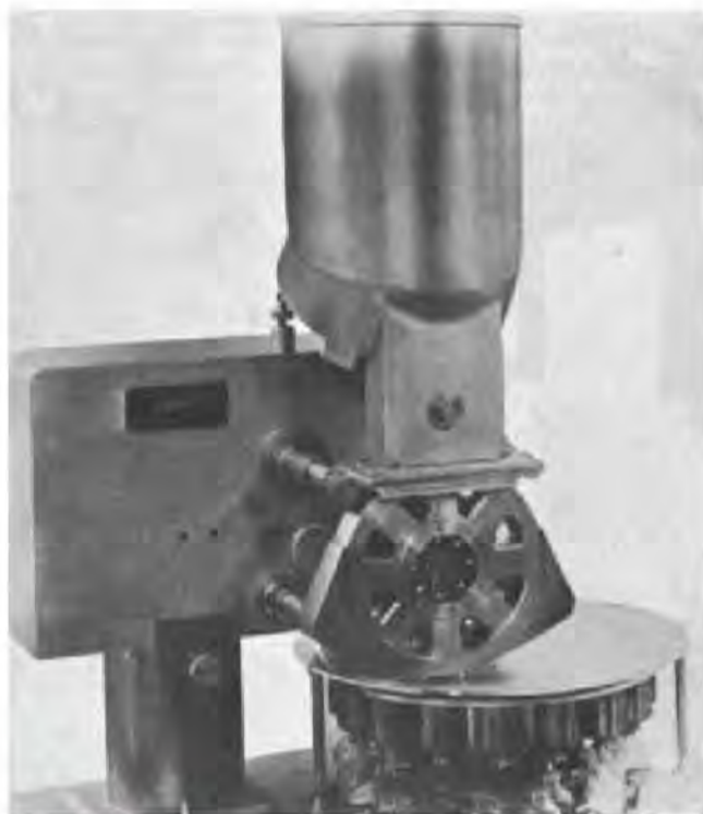
Figure 41-23. Accofil vacuum powder filler (courtesy, Perry).
