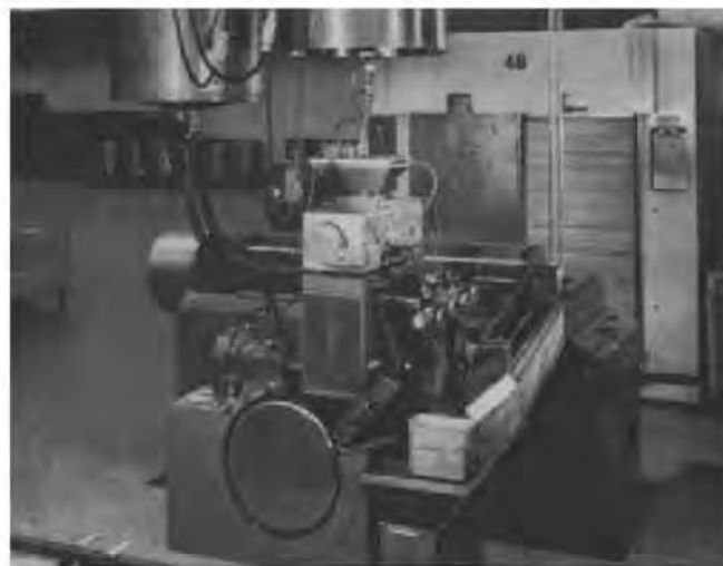
Figure 45-50. Scherer soft elastic capsule machine (courtesy, Scherer).
