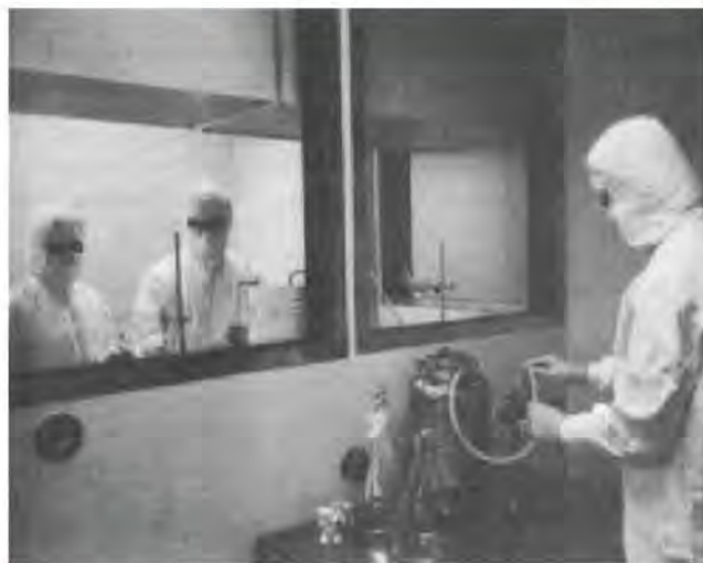
Figure 41-7. Product filtration from the aseptic staging room through a port into the aseptic filling room (courtesy, The University of Tennessee College of Pharmacy).
