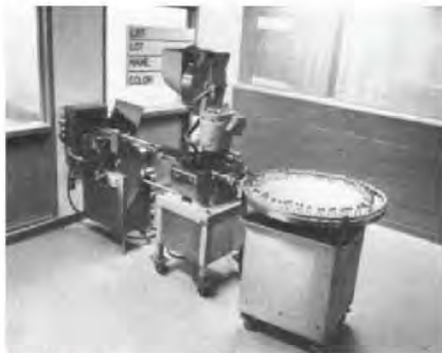
Figure 41-26. Applying aluminum caps to vials at the end of the process line (courtesy, Abbott).
