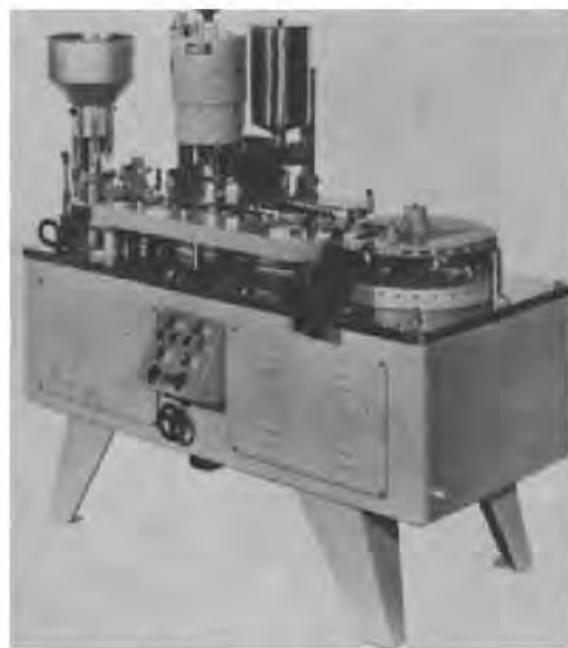
Figure 45-46. MG-2, automatic capsule-filling machine (courtesy, Supermatic).
