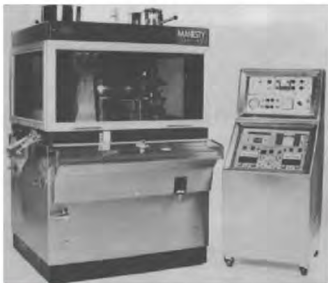
Figure 45-48. Hoefliger & Karg automatic capsule-filling machine, Model GFK 1200 (courtesy, Amaco).
