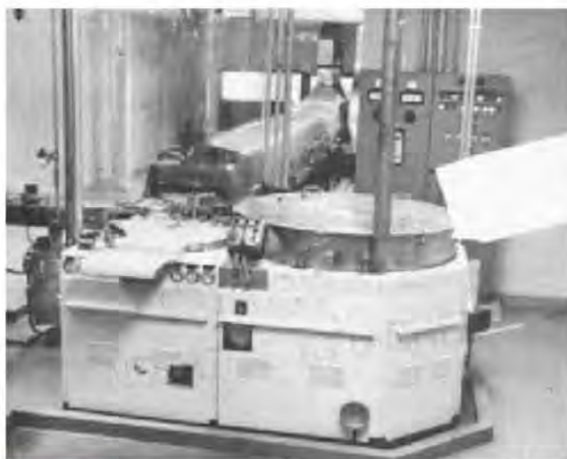
Figure 41-17. Continuous automatic line operation for vials from a rotary rinser through a sterilizing tunnel with vertical laminar-airflow protection of clean vials (courtesy, Abbott).
