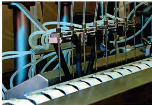
Figure 41-22. Vial filling machine, distant and close-up views (courtesy, Baxter). See Color Plate 12.
