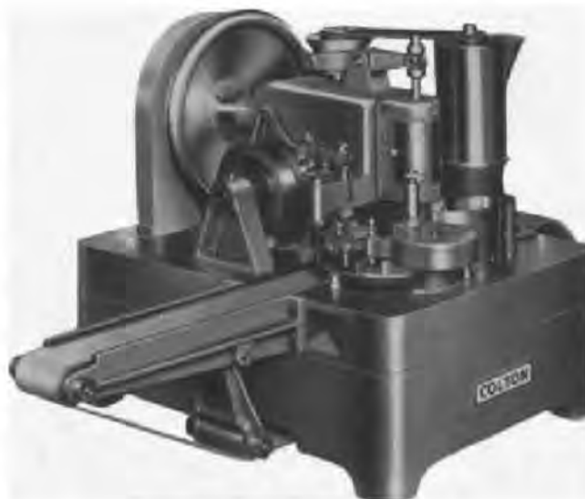
Figure 45-35. Automatic tablet triturate machine (courtesy, Vector-Colton).
