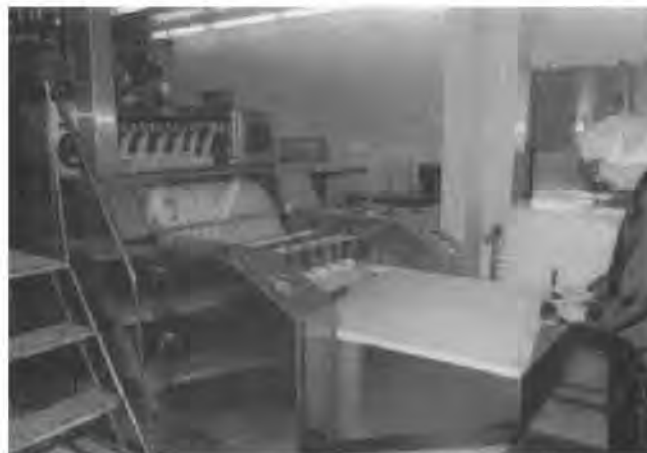
Figure 41-16. Loading end of large conveyor vial washer that subjects inverted vials to a series of cleaning steps before delivery from the far end of the washer. Note the vials in plastic blister packs at right of operator (courtesy, Merck).
