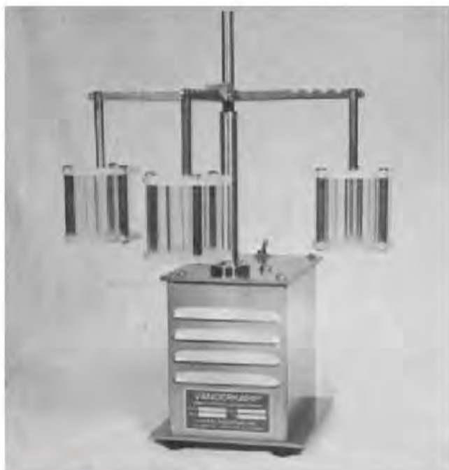
Figure 45-38. Vanderkamp tablet disintegration tester (courtesy, VanKel).
