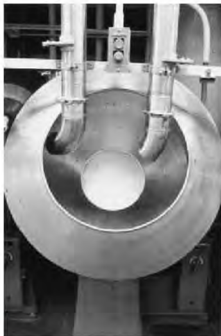
Figure 46-1. Typical equipment set-up for conventional sugar coating.
