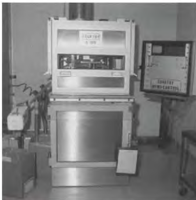
Figure 45-27. Courtoy R-100 with computer-controlled operation.
