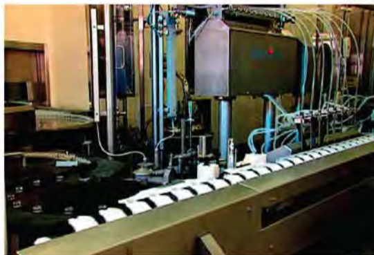
Figure 41-22. Vial filling machine, distant and close-up views (courtesy, Baxter). See Color Plate 12.
