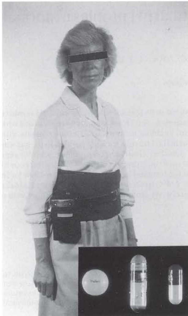
Fig. 1 The pH sensitive radiopill (inset) and portable solid state recording equipment. The aerial array is worn around the abdomen inside a cloth band.
