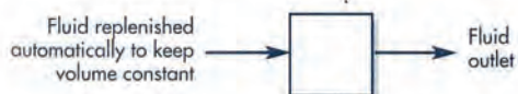
Figure 2-4. Tank with a constant volume of fluid equilibrated with drug. The volume of the fluid is 1.0 L. The fluid outlet is 10 mL/min. The fraction of drug removed per unit of time is 10/1000, or 0.01 \text{ min}^{-1} .
