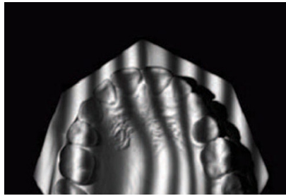
Fig. 2 Digital fringe projection on a dental model 35
