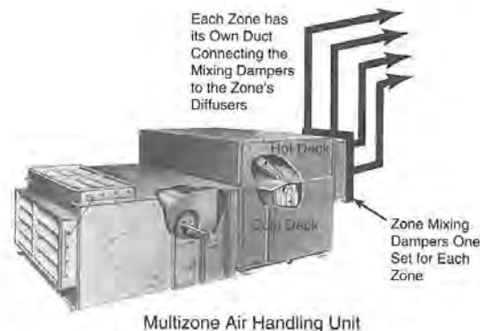
Figure 24.1 Multizone Dampers
