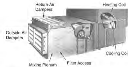
Figure 2.1 Air Handling Unit
