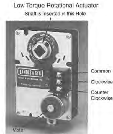
Figure 3.7 Rotational Actuator
