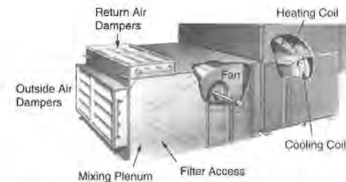
Figure 2.1 Air Handling Unit
