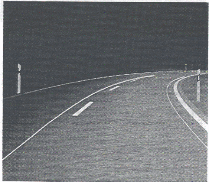
Fig. 8: Control of the headlamps with path prediction
