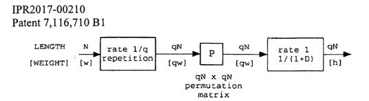
Figure 3. Encoder for a (qN, N) repeat and accumulate code. The numbers above the input-output lines indicate the length of the corresponding block, and those below the lines indicate the weight of the block.
