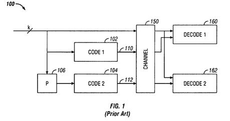
Figure 1 is a schematic diagram of a prior "turbo code" system. *Id.* at 2:14–15. The '710 patent specification describes Figure 1 as follows:
