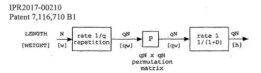
Figure 3. Encoder for a (qN, N) repeat and accumulate code. The numbers above the input-output lines indicate the length of the corresponding block, and those below the lines indicate the weight of the block.
