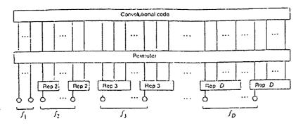
Figure 2: A general *irregular turbocode*. For d = 1, ..., D, fraction  $f_d$  of the codeword bits are repeated d times, permuted and connected to a convolutional code.
