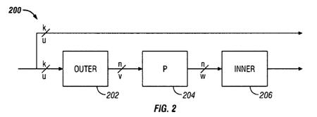
Figure 2 of the '710 patent is a schematic diagram of coder 200. *Id*. at 2:16–17.
