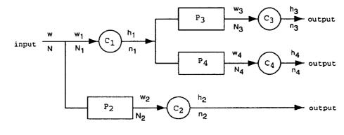
Figure 1. A "turbo-like" code with  $s_1 = \{1, 2\}, s_0 = \{2, 3, 4\}, \overline{s}_0 = \{1\}.$
