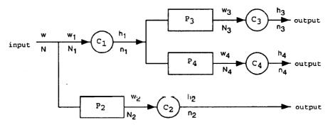
Figure 1. A "turbo-like" code with  $s_{1} = \{1, 2\}, s_{0} = \{2, 3, 4\}, \overline{s}_{0} = \{1\}.$
