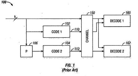
Figure 1 is a schematic diagram of a prior "turbo code" system. *Id.* at 2:14–15. The '710 patent specification describes Figure 1 as follows:
