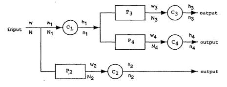
Figure 1. A "turbo-like" code with  $s_I = \{1, 2\}, s_O = \{2, 3, 4\}, \overline{s}_O = \{1\}.$
