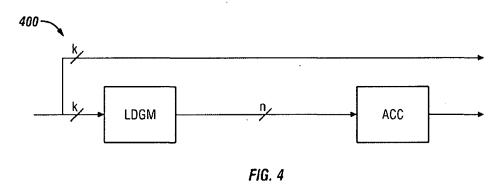
Figure 4 of the '710 patent is a schematic of an irregular repeat and accumulate coder using a low density generator matrix  $(LDGM)^2$  coder. *Id.* at 2:20–21, 3:25. The LDGM coder "performs an irregular repeat of the k bits in the block, as shown in FIG. 4." *Id.* at 3:52–54. LDGM codes are a special class of low density parity check codes that allow for less encoding
