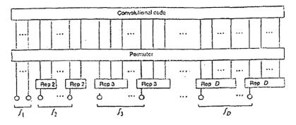
Figure 2: A general *irregular turbocode*. For d = 1, ..., D, fraction  $f_d$  of the codeword bits are repeated d times, permuted and connected to a convolutional code.
