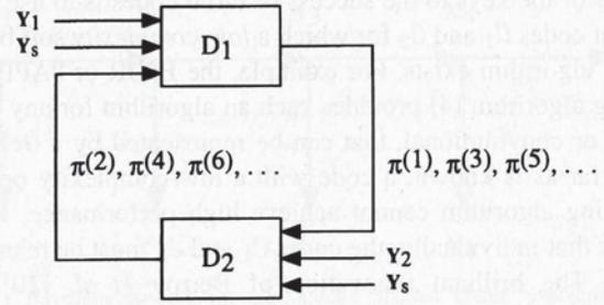
Fig. 3. Block diagram of turbo decoding procedure.
