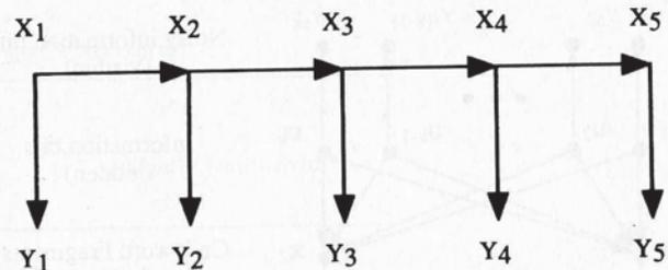
Fig. 6. Bayesian network for the "hidden Markov chain" problem. Here,  $X_1, \dots, X_N$  form a Markov chain, and  $Y_1, \dots, Y_N$  are noisy versions of  $X_1, \dots, X_N$ . The problem is to compute the conditional probabilities of the hidden variables  $X_i$  based in the "evidence" variables  $Y_i$ .
