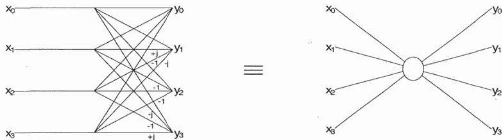
Figure 2.4 The radix-4 butterfly.
