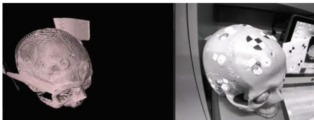
Figure 2. Graphical display. Right image shows real video output from one Micron camera, while the overlaid model of the skull, after registration, is depicted on the left.
