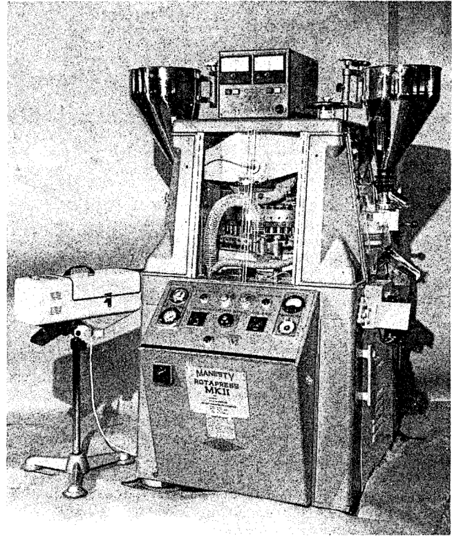
Fig. 89-26. Mark II Rotapress with 61 stations, equipped with deduster (left) and the Thomas Tablet Sentinel (top of press) (courtesy, Thomas/Manesty).
