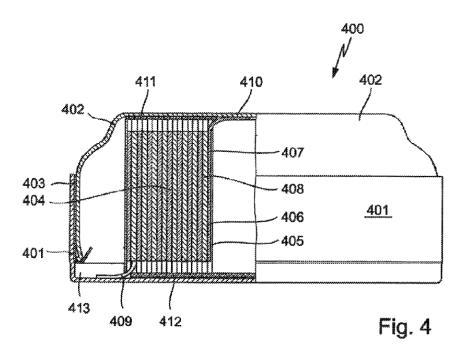
Figure 4 of the '913 patent, above, shows button cell 400 including a housing comprising cup part 401 and top part 402, with seal 403 arranged therebetween, and an assembly of electrodes 407 and 408 and separators 405
