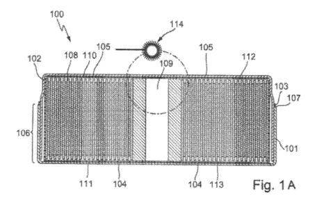
Figure 1A of the '858 patent, above, shows button cell 100 comprising two metal housing halves, metal cup part 101 and metal top part 102, that form plane bottom region 104 and plane top region 105; electrode assembly 108 wound on winding core 109; metal foil output conductors 110 and 111; and insulating elements 112 and 113. *Id.* at 6:52–7:18, Fig. 1A.
