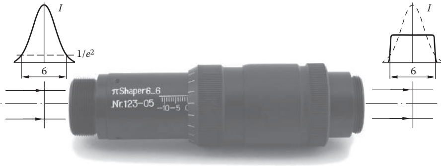
FIGURE 7.21 Refractive field mapping beam shaper, \pi Shaper. (Reproduced from Laskin, A., Williams, G., and Demidovich, A., Applying of refractive beam shapers in creating spots of uniform intensity and various shapes, in Laser Resonators and Beam Control XII , Kudryashov, A. V., Paxton, A. H., and Ilchenko, V. S., eds., SPIE, Bellingham, WA, 2010. With permission.)
