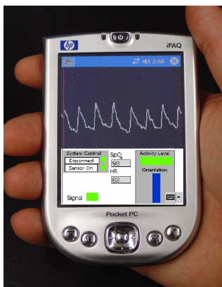
Fig. 3. Sample PDA Graphical User Interface (GUI).
