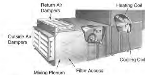
Figure 2.1 Air Handling Unit
