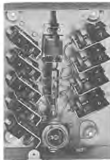
Figure 6.12 Stepping switch. (Courtesy of Johnson Controls Inc.)
