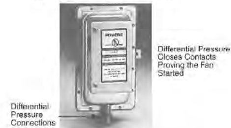
Figure 13.6 Binary Input Status Hardware Point
