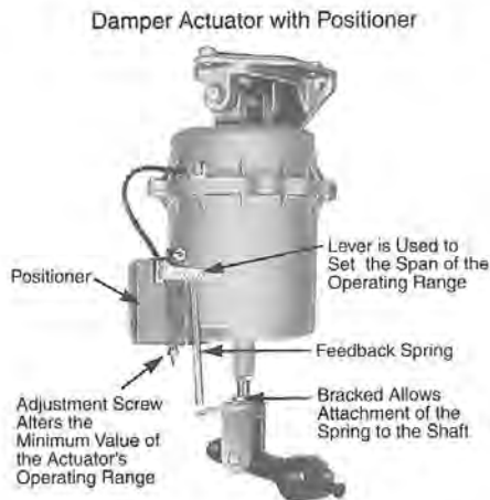
Figure 10.3 Positioning Relay and Damper Actuator
