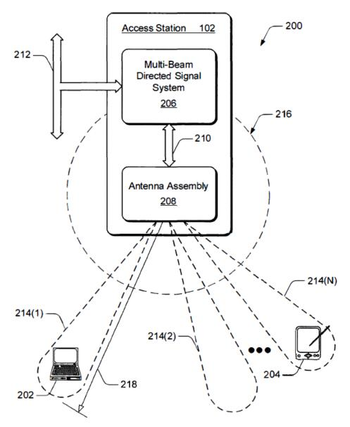
As shown, "antenna assembly 208 can be implemented as two or more antennas . . . to emanate multiple directed communication beams 214(1), 214(2), . . . , 214(N)." Ex. 1001, 4:54–57. "[C]lient device 202 can communicate via directed communication beam 214(1) with a first channel of the multi-beam directed signal system 206, and client device 204 can communicate via directed communication beam[] 214(N) with a second channel of the multi-beam directed signal system 206." *Id.* at 5:16–21.
