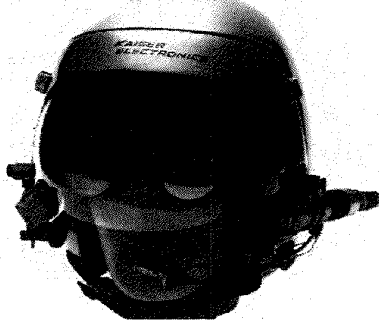
FIG. 4.1. Optical see-through head-mounted display. (Photo courtesy of KaiserElectro-Optics.)
