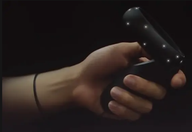
Facebook's VR controllers are tracked via infrared LEDs under the plastic
