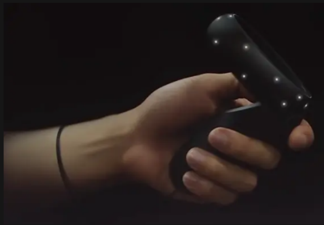
Facebook's VR controllers are tracked via infrared LEDs under the plastic
