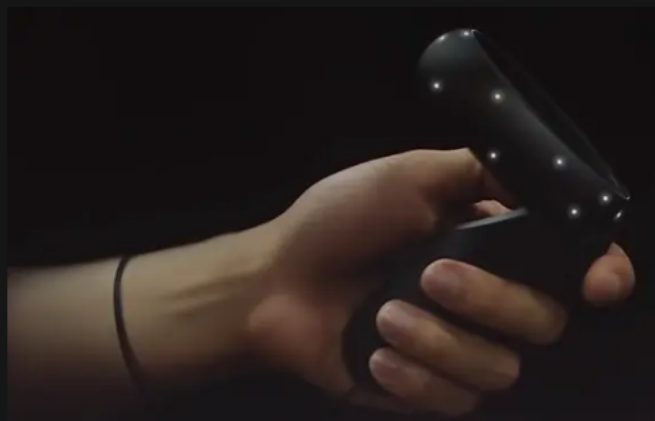
Facebook's VR controllers are tracked via infrared LEDs under the plastic
