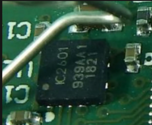
The IMU in the current Touch controllers for Rift S and Quest
