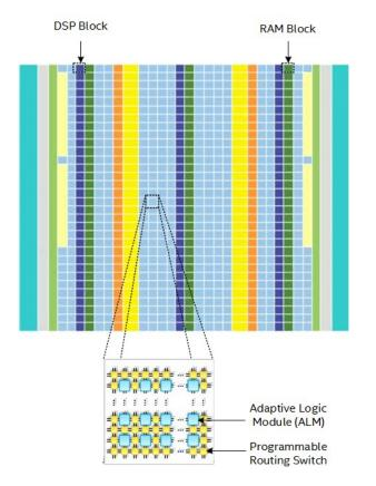
When software is "executed" on the FPGA, it is not executing in the same sense that compiled and assembled instructions execute on CPUs and GPUs. Instead, data flows through customized deep pipelines on the FPGA that match the operations expressed in the software. Because the dataflow pipeline hardware matches the software, control overhead is eliminated, which results in improved performance and efficiency.
