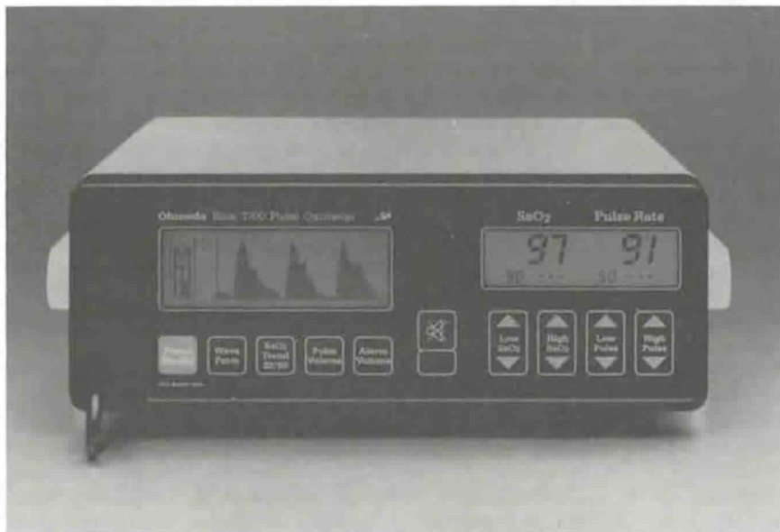
Figure 12.2 Front panel of Ohmeda Biox 3700 pulse oximeter (Courtesy of Ohmeda). The display at the left side shows real-time waveforms and pulse strength, while the display at the right side is used for alarm settings.
